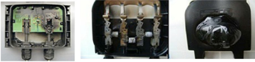
Figure 5. Junction box faults (Mellit et al. 2018)
