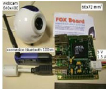
Figure 7. Sensor implemented using the fox board.
